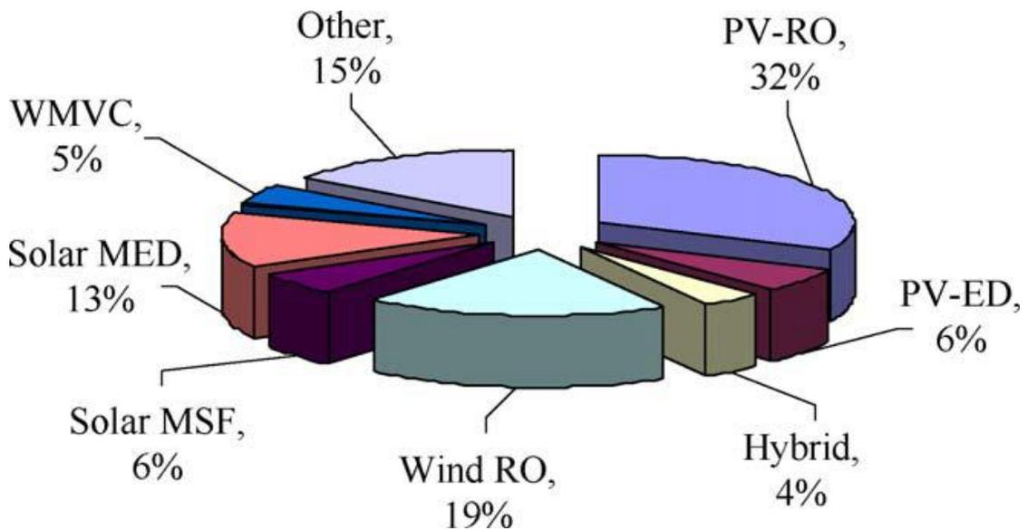
Figure 16: Distribution of renewable energy powered desalination technologies [14]
