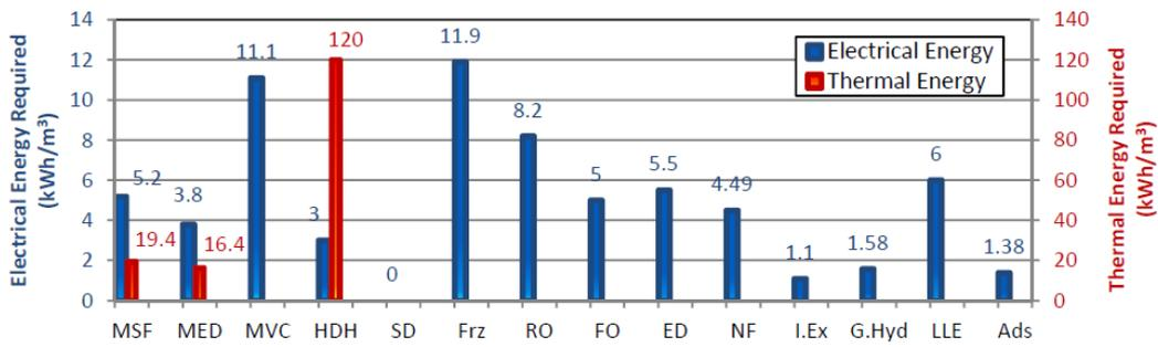
Figure 26: Amount of energy required for different desalination technologies [6]
