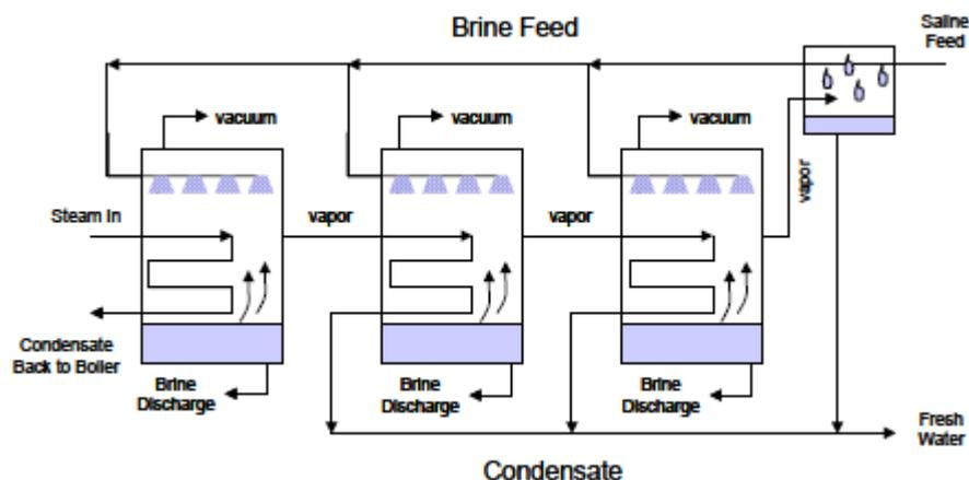
Figure 6: Schematic of a Multi Effect Distillation plant [7]
