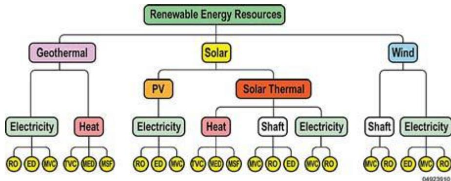
Figure 17: Combinations of Renewable Energy Sources with desalination technologies [8]
