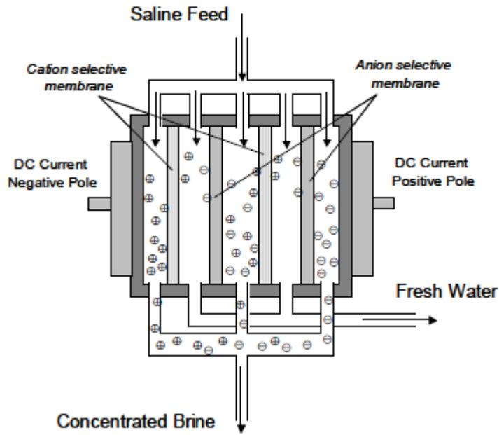
Figure 9: Schematic of Electrodialysis desalination plant [7]
