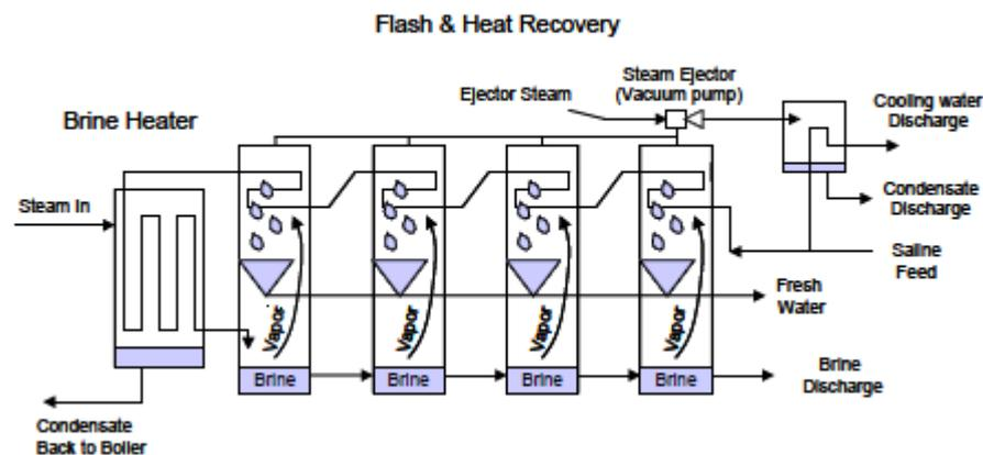
Figure 5: Schematic of Multi Stage Flash desalination process [7]
