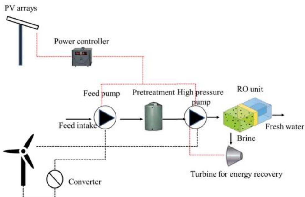
Figure 23: Schematic diagram of a solar and wind driven Reverse Osmosis system [20]
