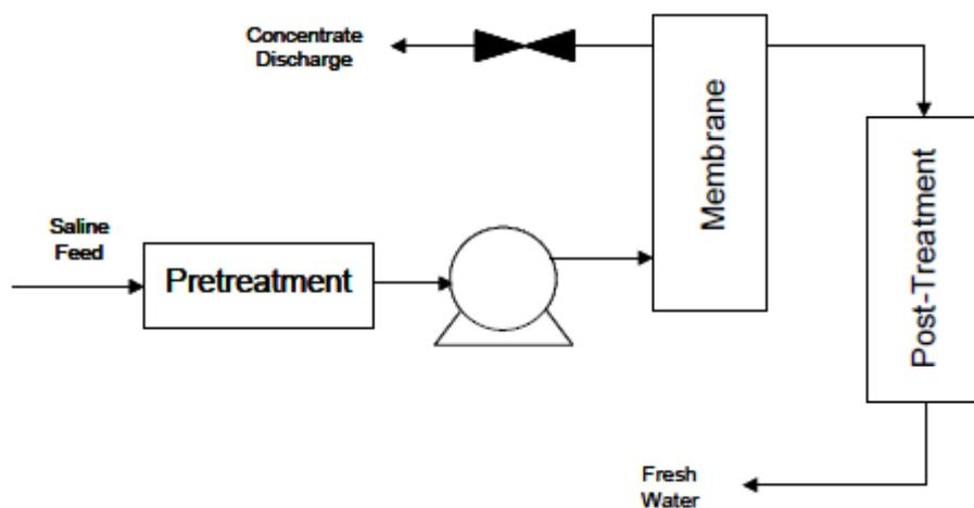
*Figure 8: Schematic of Reverse Osmosis desalination plant [7]*
