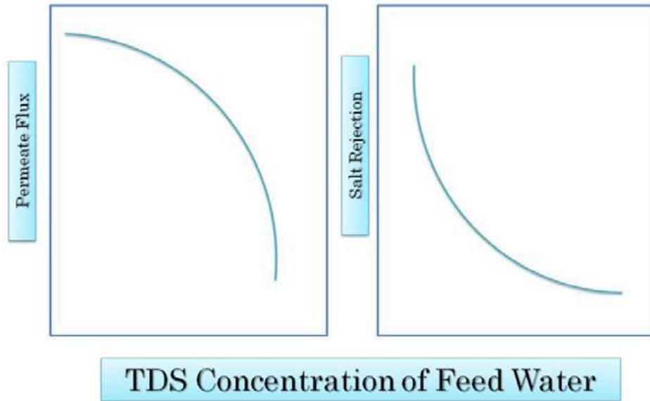
Figure 35: Effect of feedwater salinity in Reverse Osmosis desalination [18]
