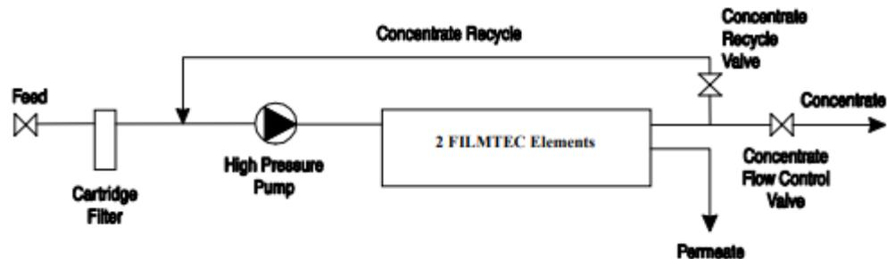
Figure 40: Single module Reverse Osmosis system [22]
