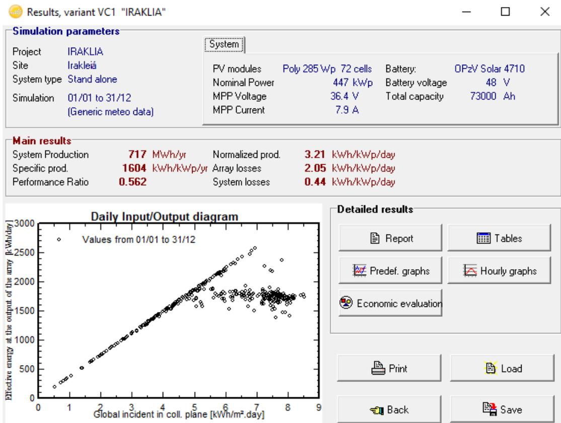
No back-up generator is used, for reasons of simplicity. All the system's losses and efficiencies were calculated by default by the program.
