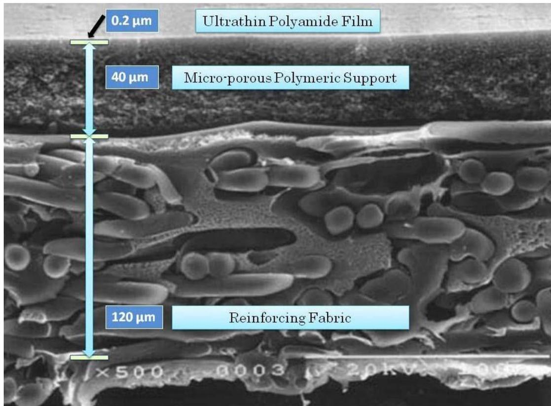
Figure 31: Structure of a RO membrane [15]
