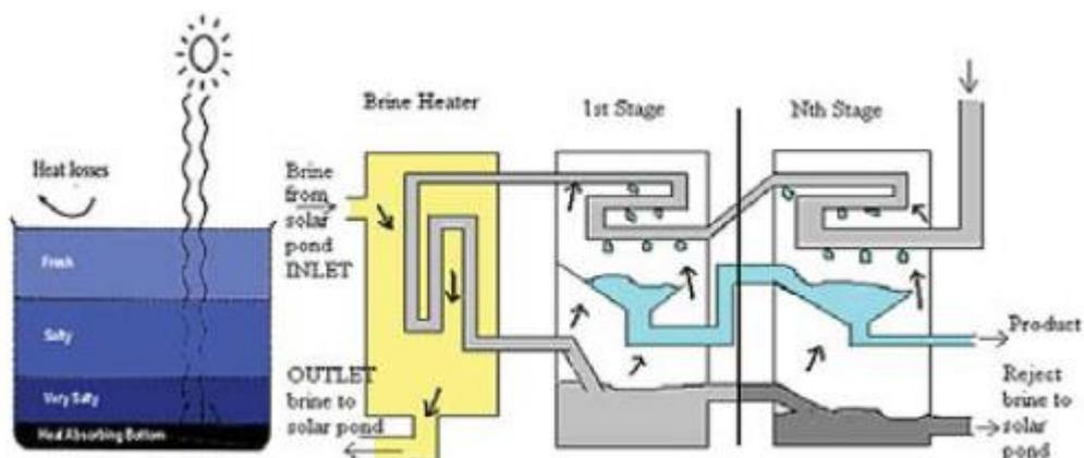
Figure 20: Solar pond assisted desalination [8]
