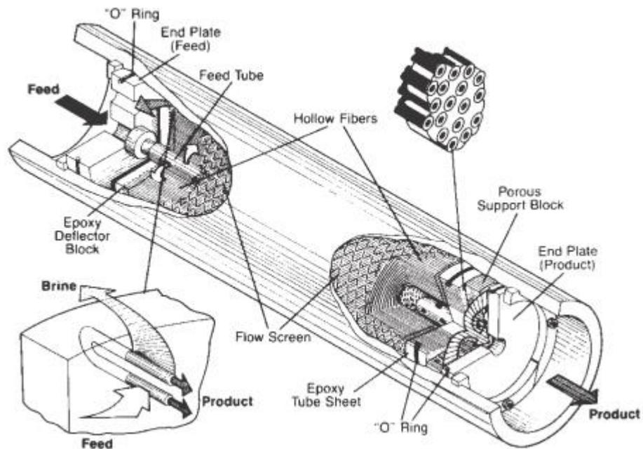
Figure 32: Hollow-fiber membrane configuration [16]
