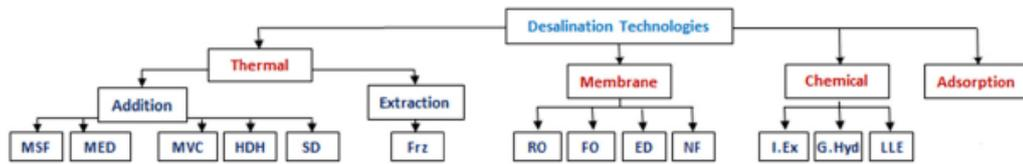
Figure 4: Classification of desalination technologies [6]
