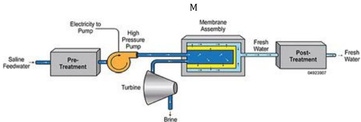
Figure 30: Reverse Osmosis Desalination system [8]
