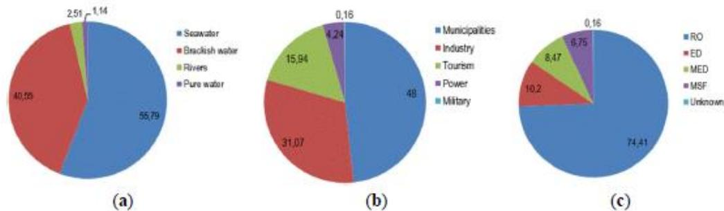
Figure 15: Desalinated water production in Greece according to: a) Feedwater, b) the use of fresh water, c) the used technology [9]
