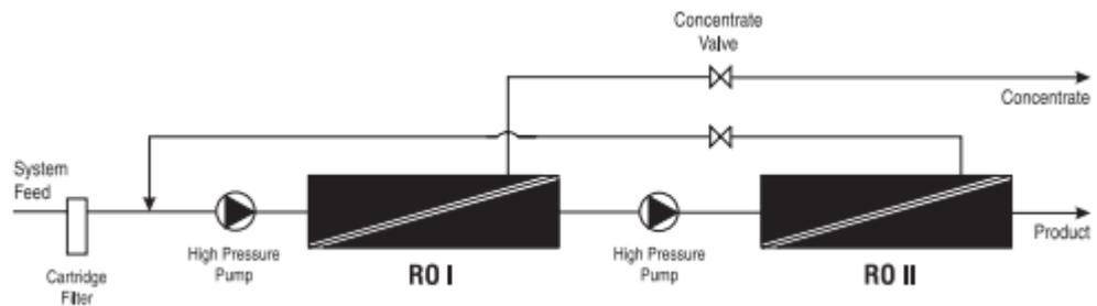
Figure 43: Permeate staged reverse osmosis system [22]
