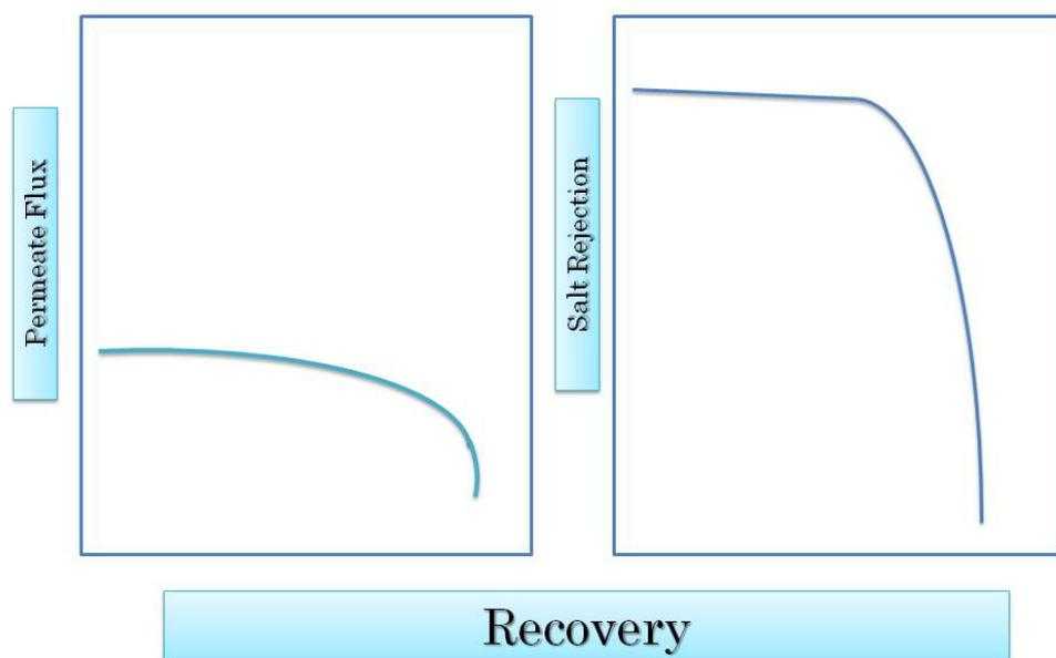
Figure 36: Effect of recovery in Reverse Osmosis desalination [18]
