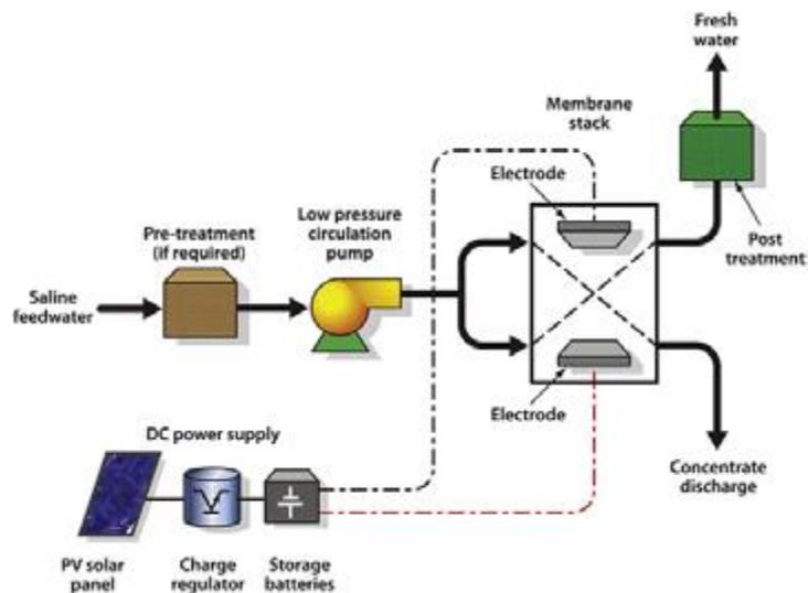
Figure 21: PV powered Electrodialysis desalination system [8]
