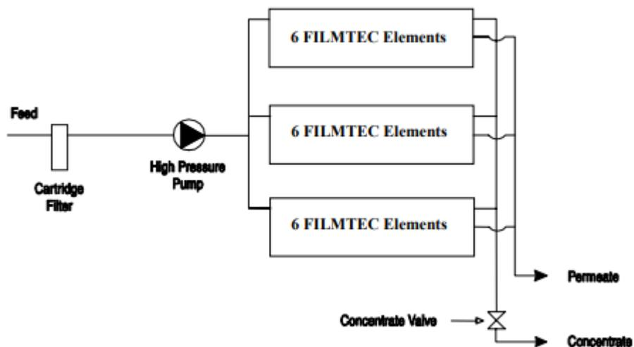
Figure 41: Single-stage, multiple module reverse osmosis system [22]
