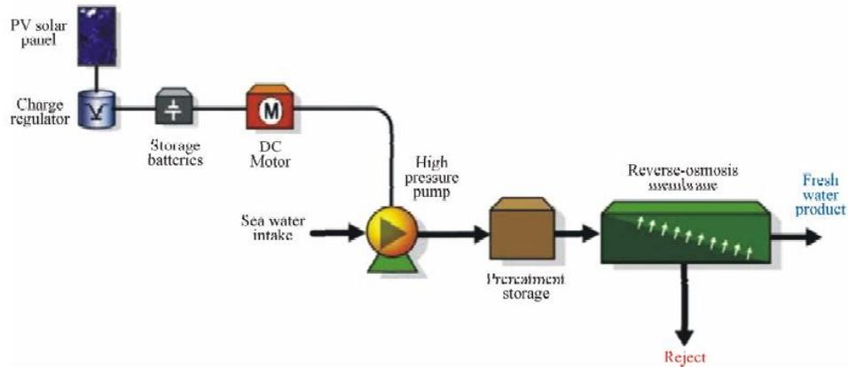
Figure 37: Schematic of a PV powered RO desalination system
