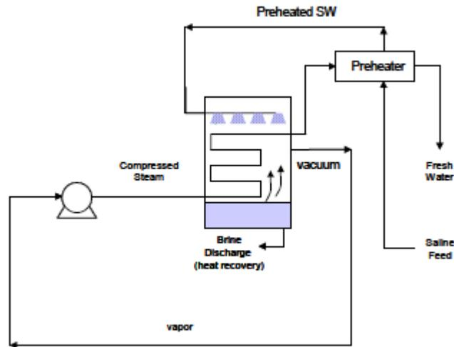
Figure 7: Schematic of Vapor Compression desalination [7]
