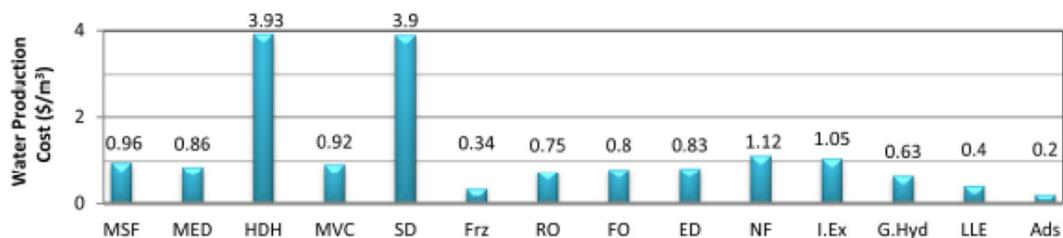
Figure 25 : Water production costs of different desalination technologies [6]
