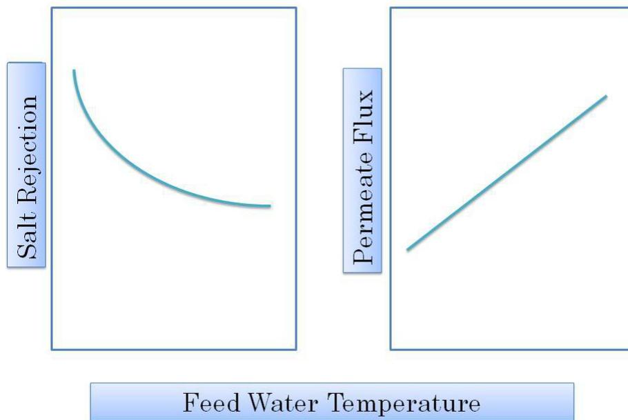
Figure 34: Effect of temperature in Reverse Osmosis desalination [18]
