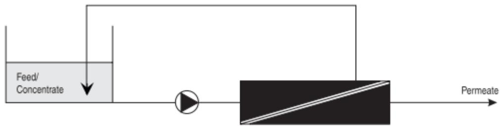
Figure 39: Batch Reverse Osmosis process [22]
