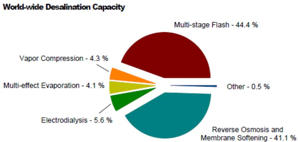
Figure 14: Global distribution of installed desalination capacity by technology [7]
