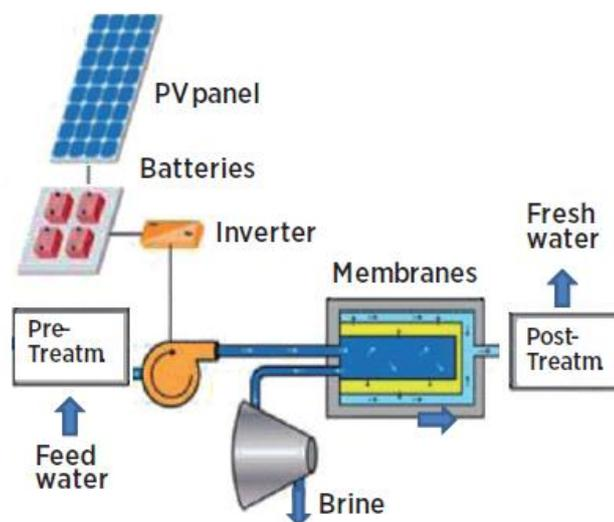
Figure 22: Coupled PV and RO desalination plants [13]
