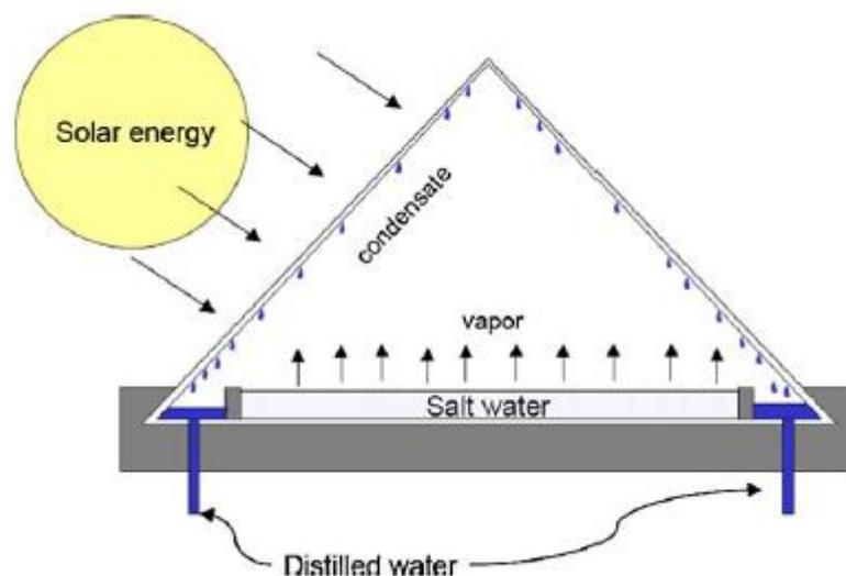
Figure 18: The basic design of a solar distillation unit [14]
