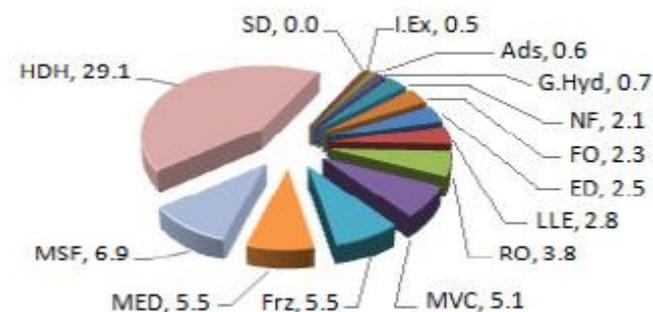
Figure 27: Amount of released CO<sub>2</sub> for different desalination technologies, kg/m<sup>3</sup> [6]
