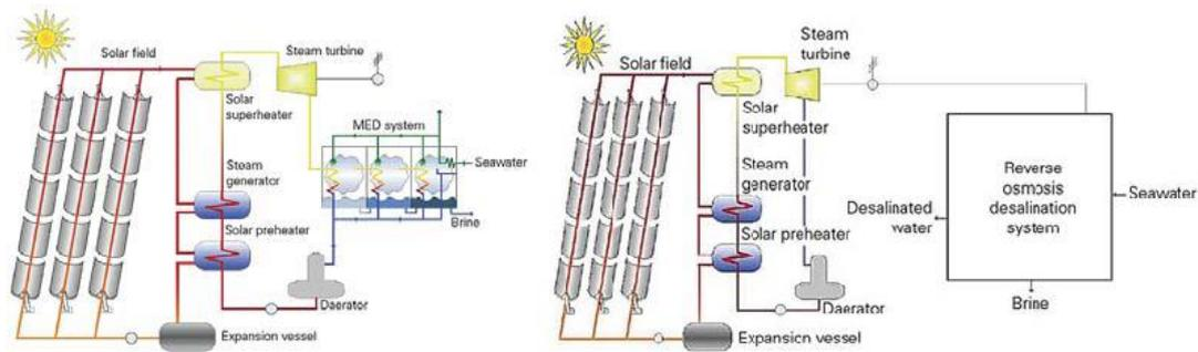
Figure 19: CSP power plant couple with MEB and RO desalination unit [8]
