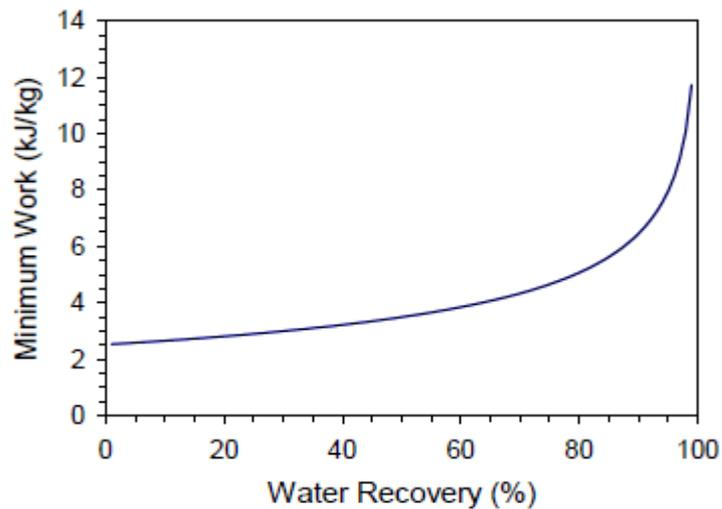
Figure 10: The theoretical minimum energy for desalination of seawater as function of freshwater recovery [7]
