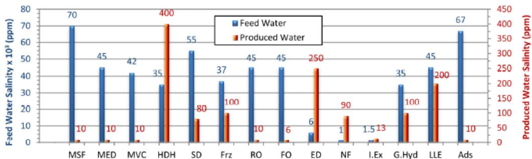
Figure 24: Capability of different desalination systems regarding salinity of feed and produced water, ppm [6]
