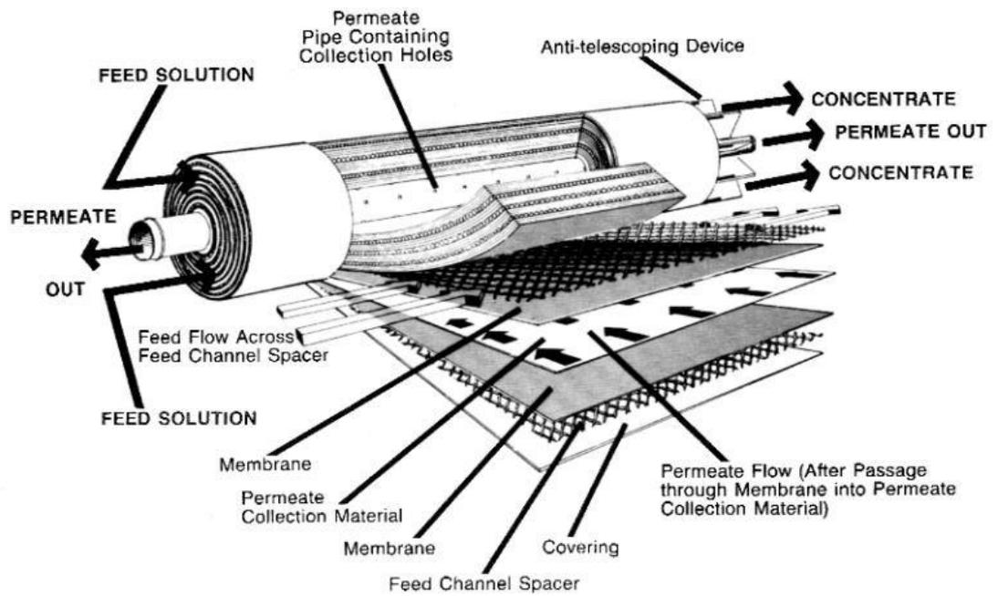
Figure 33: Spiral-wound membrane configuration [16]
