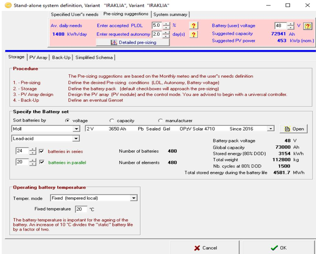
The PV module chosen is a generic 285Wp 30V, Si-poly module from the database. A simple DC-DC controller is used, as it is cheaper and the PV array results in 1568 modules covering an area of 3042m<sup>2</sup>.
