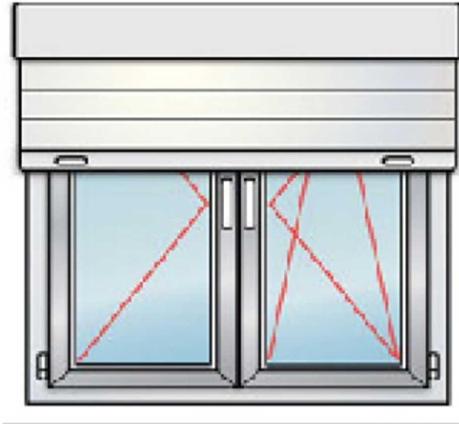
Figure 18: Double Opening Window Design (Source: www.etoimokoufoma.spatharakis.gr )
