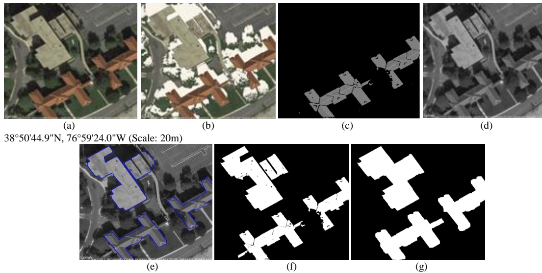
Figure 19: All stages for building detection in satellite images
