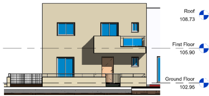
Figure 55: P 2 – South Elevation
