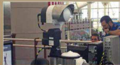
The PTU-D300 is a key component in Gineq's stand-off detection system for the TSA.
