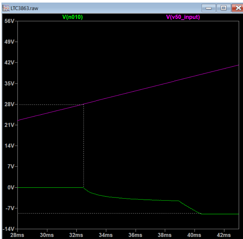
Figure 17. DC DC inverter activation at 28V
