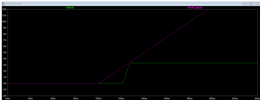
Figure 14. Buck converter Activation
