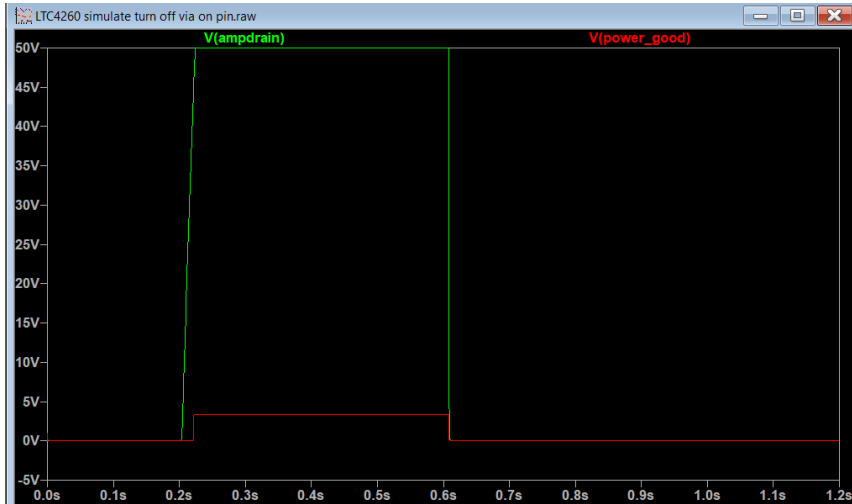
Figure 31: Behavior of "Power Good" Pin
