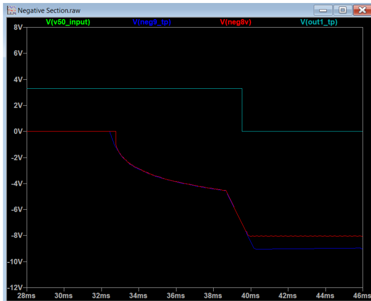
Figure 24. Negative Voltage Fault has been released.
