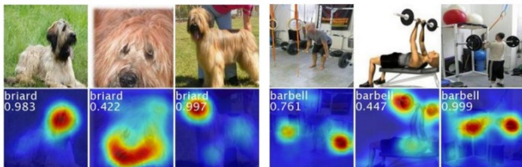
Figure 12. The CAMs of two classes from ILSVRC (Russakovsky O., 2015: 211). The maps highlight the discriminative image regions used for image classification, the head of the animal and the plates in barbell (Zhou B., 2016, 2921).
