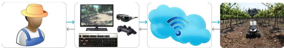
Figure 4. Robot teleoperation scheme in the case of the agricultural robot sprayer
