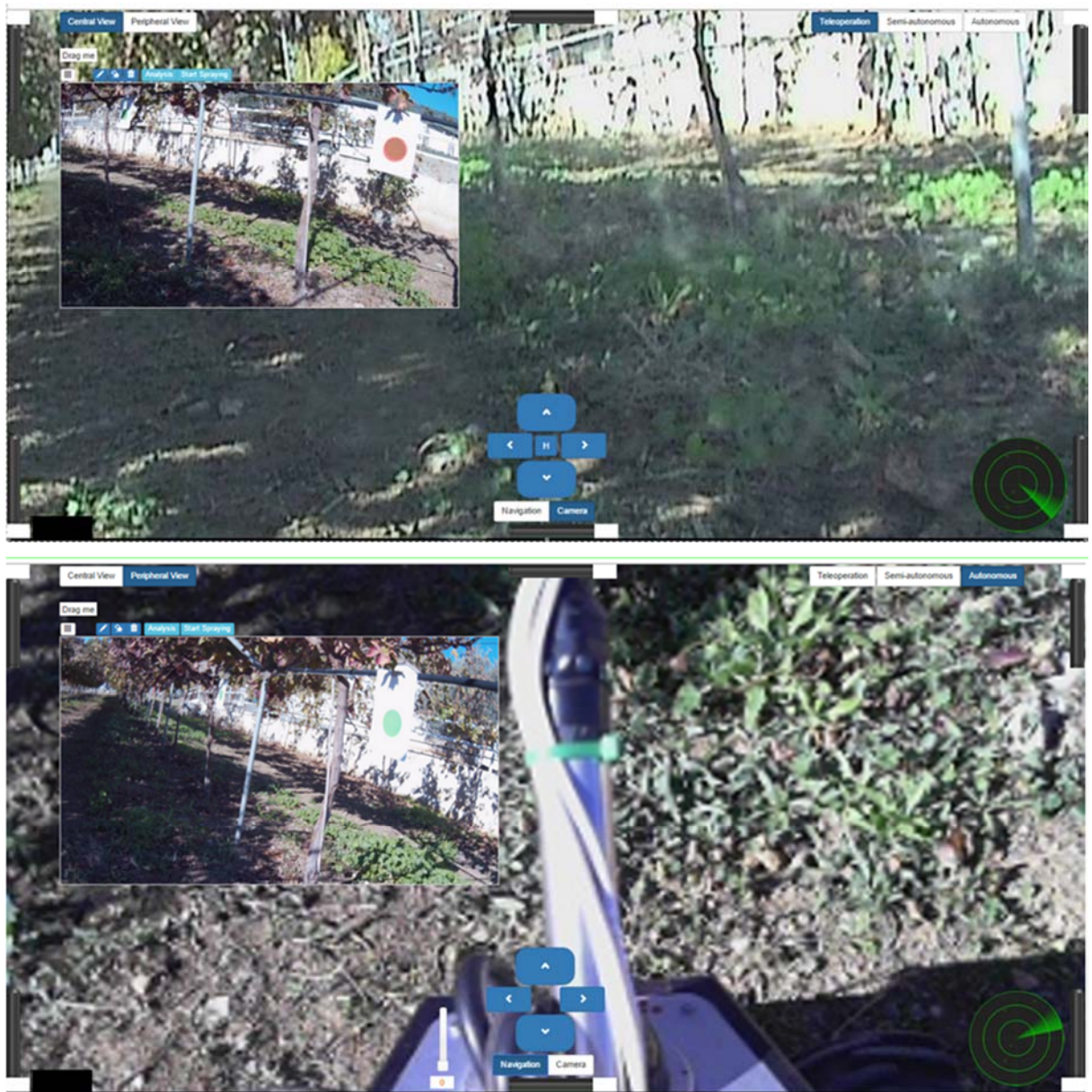
Figure 16. The SAARS user interface - Top: Central camera view, Bottom: Peripheral camera view
