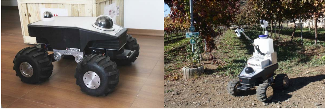
Figure 17. Left: The Summit XL mobile platform, Right: the transformed agricultural robot sprayer
