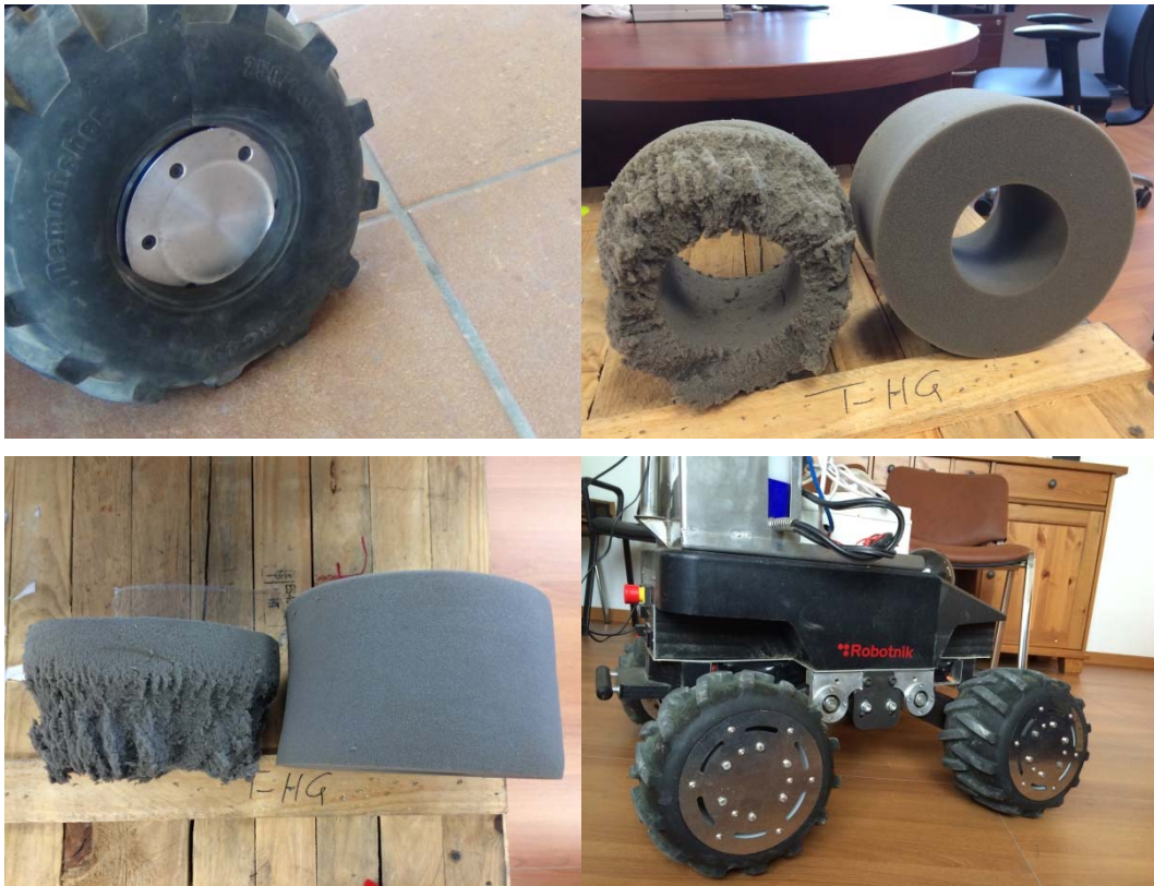
Figure 12. Problem with robot wheels – Top-left: the damaged wheel, Top-right and bottom-left: the damaged inside soft foam (on the left, the original soft foam on the right); Bottom-right: the new set of wheels with hard foam inside.
