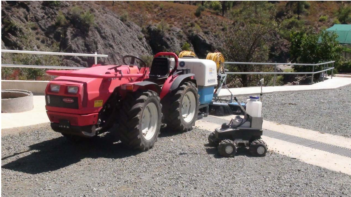
Figure 26. Left a tractor sprayer, Right: the AgriRobot sprayer
