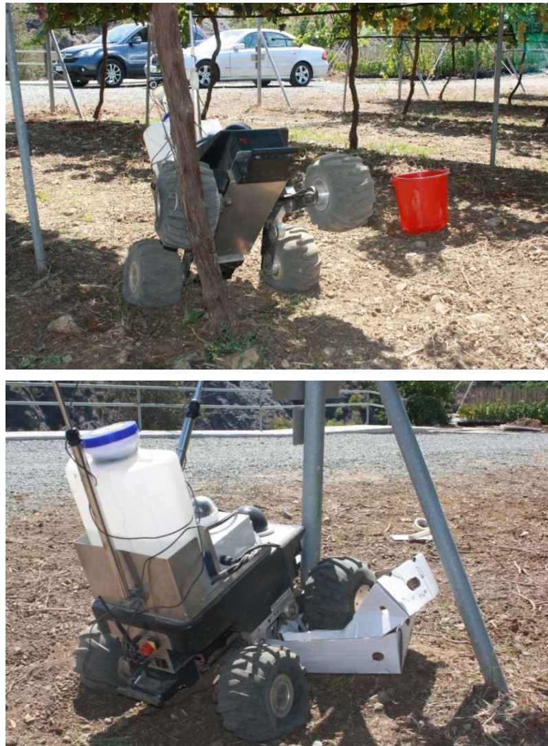
Figure 6. Top: Collision of the AgriRobot on a vine tree stem; Bottom: Collision on a fruit-collection box (obstacle) and on a pole
