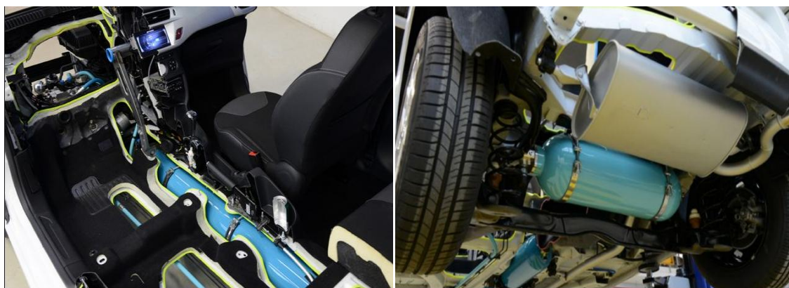
Compressed Air Cylinder position
