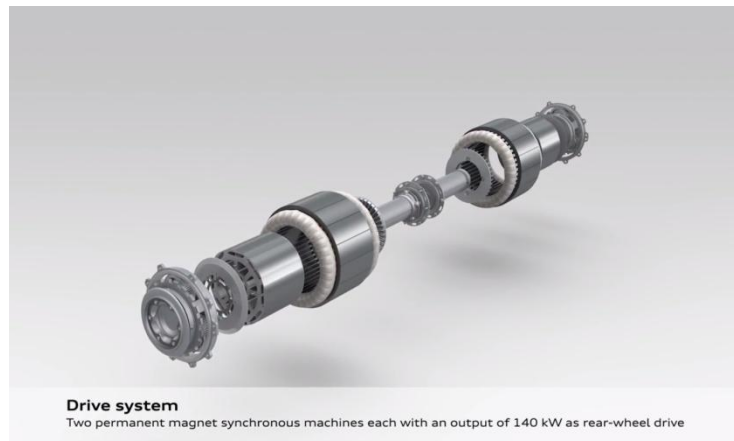
Drive system of two permanent magnet of R8
