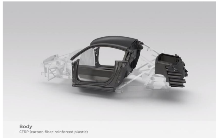
Body frame R8 with CFRP
